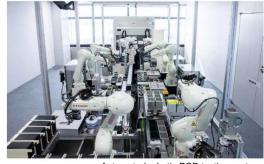
Automated robotic PCR testing system
