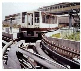
Kawasaki Computer-controlled Vehicle (KCV) system test line
